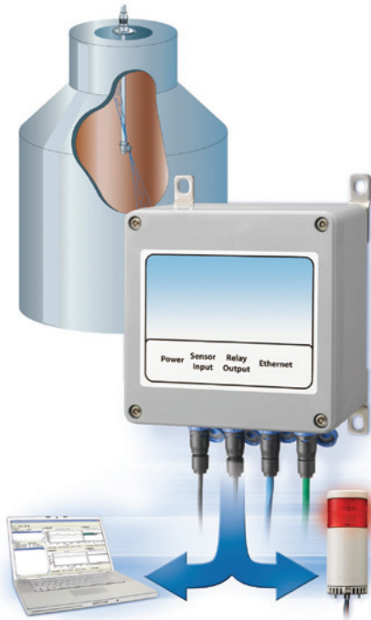
Figure 5. Unit mounted on outside of vessel detects loss of rotation and variations in rotation speed and fluid pressure.
