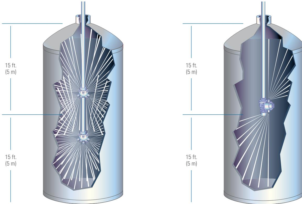
Spray distance is usually expressed in terms of tank diameter. If your tank is 15 ft. (5 m) in diameter and 30 ft. (9 m) tall, you will need two tank cleaners that can clean 15 ft. (5 m) or one that can clean up to 30 ft. (9 m).
