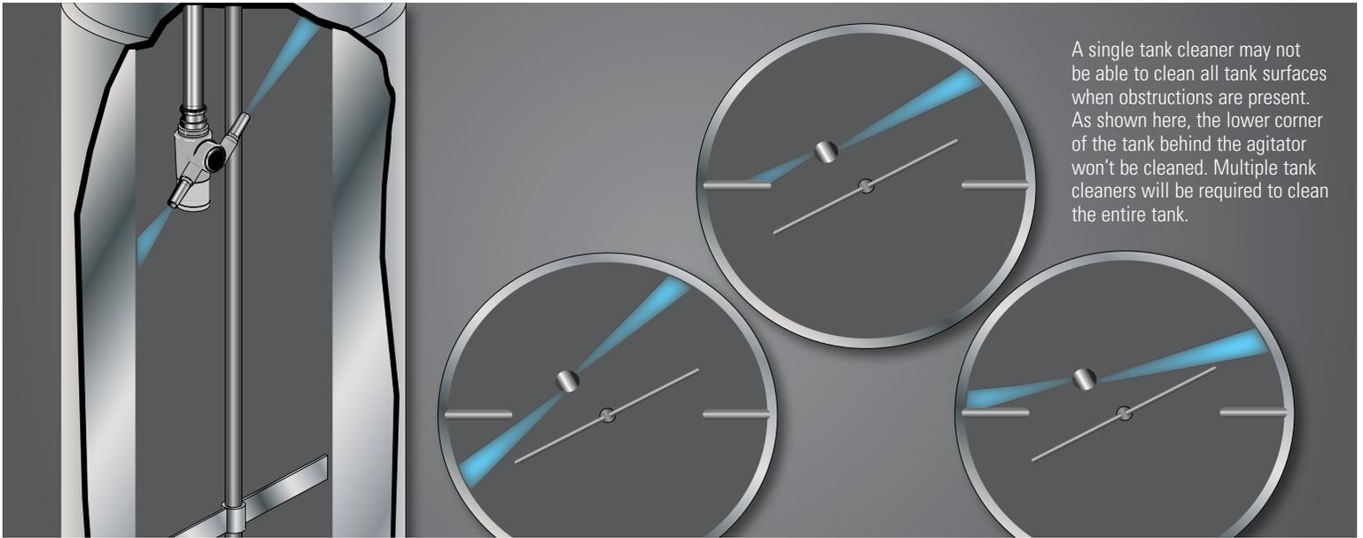
A single tank cleaner may not be able to clean all tank surfaces when obstructions are present. As shown here, the lower corner of the tank behind the agitator won't be cleaned. Multiple tank cleaners will be required to clean the entire tank.
